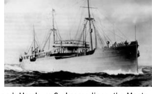
kW each at 140 rpm. On the other hand, **Hamburg Sud** cargo liner, the Monte Penedo, is the first ship to be powered by two stroke engine. The two **Sulzer**
